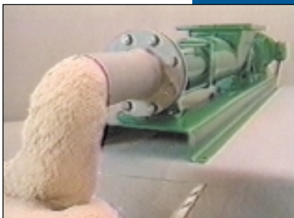
NEMO NM SF Pump used to transport bread dough
